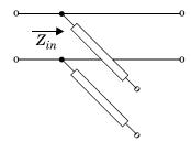
$Z_{in}\,$  is the input impedance of the shunt circuit. The ABCD-parameters for the shunt stub are calculated as
