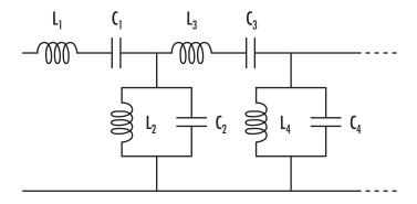
Where  $[L_1, L_2, L_3, L_4, ...]$  is the value of the 'L' property, and  $[C_1, C_2, C_3, C_4, ...]$  is the value of the 'C' property.
