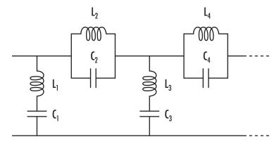
Where  $[L_1, L_2, L_3, L_4, ...]$  is the value of the 'L' property, and  $[C_1, C_2, C_3, C_4, ...]$  is the value of the 'C' property.
