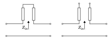
$Z_{in}\,$  is the input impedance of the series circuit. The ABCD-parameters for the series stub are calculated as
